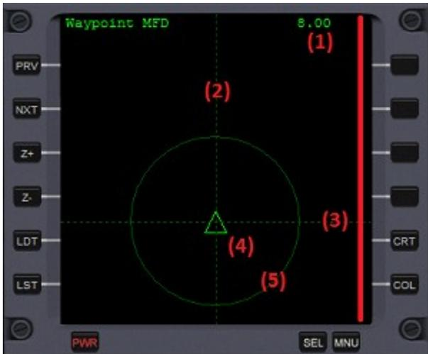
(1) Zoom - The distance from the bottom of the MFD to the top. This distance is marked by the red line on the right.
