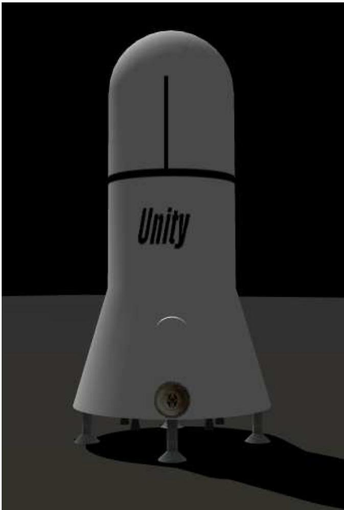
Unity is a lunar spacecraft which can hold 28,000 kg of LH2/LOX propellant. It also has enough living space for six crew/passengers to comfortably work and rest during the four-day trip to the moon.
