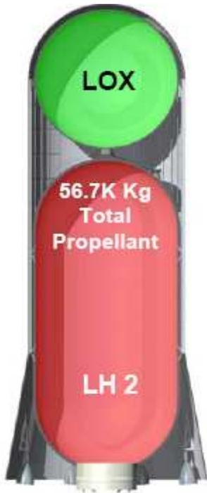
The Tanker is basically a Unity with no hab area or landing legs. The space that would be taken up by a hab area is used to house a fuel tank that is twice as big as the Unity's. The Tanker holds a whopping 56,700 kilograms of LH2/LOX propellant.
