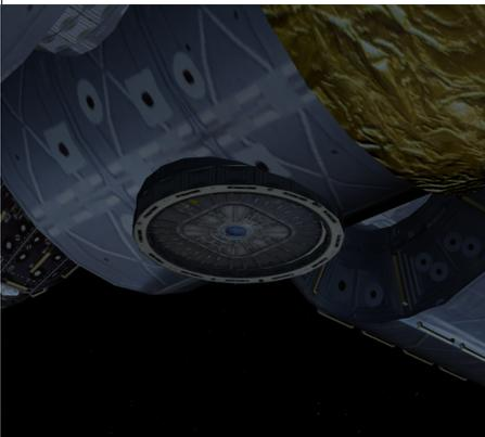
Located at the bottom of the module where the PMA adapters for Docking Ports #1 and 3 are docked to Docking Port #6. This docking port does not currently have an use, though it can be used to dock compatible ships and/or new modules.
