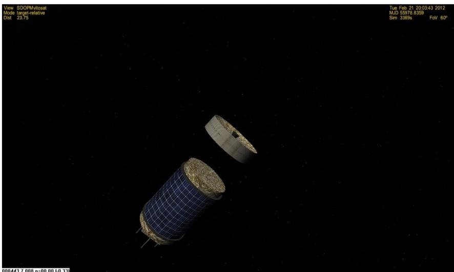
The OPM is used for the final orbit insertion after the second stage release. With its single 200 000 N engine and its 5000 kg of fuel it can send a satellite of 12 tonnes at 2000 km of altitude. It's a spacecraft3 vessel.
