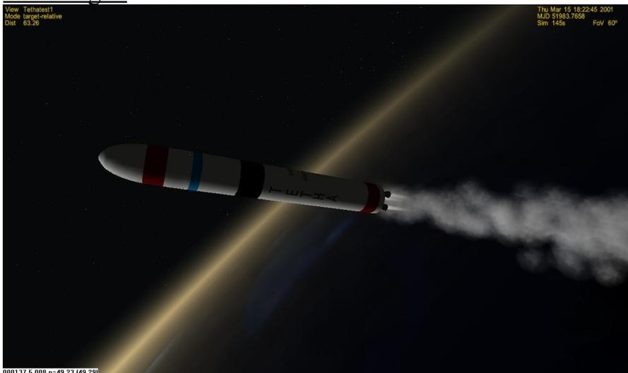
It's the first ignited stage during the launch. It have 3 engine with a power of 2 800 000 N available during 4 minutes et 21 seconds.
