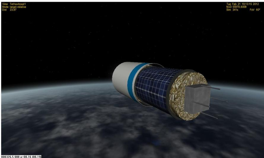
The second stage is burned after the first stage release. It has 1 engine of 730 000 N available during 2 minutes.
