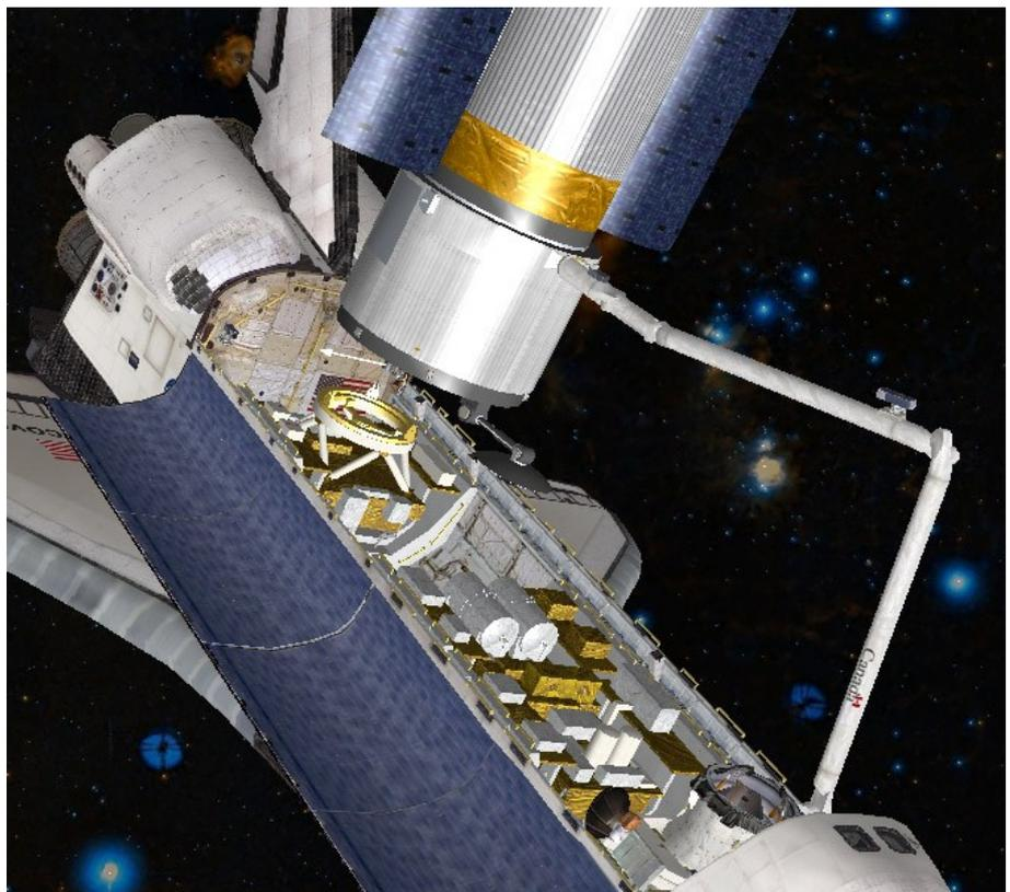
Align the docking pins on KH-12 with the docking latches then release KH-12 from the RMS arm.
