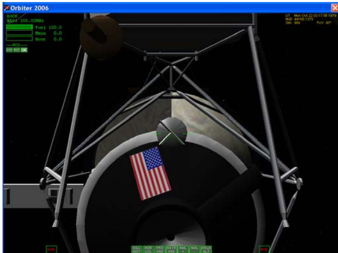
Figure 3-1a TRS Docking - cockpit view. Note how the green Docking HUD marker aligns with Skylab's docking target. The red portion of the target concealed, indicating proper alignment.
