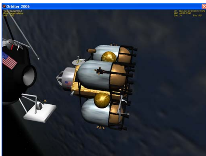
Figure 3-1b TRS Docking - external view. The extended TV camera (above and aft of the grapple fixture) lines up with the docking target.
