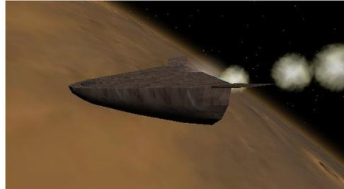
The Aeroneutronic lander was a lifting-body design which landed on its tail; a parachute helped with the problematic transition from forward to tail-first-downward flight.
