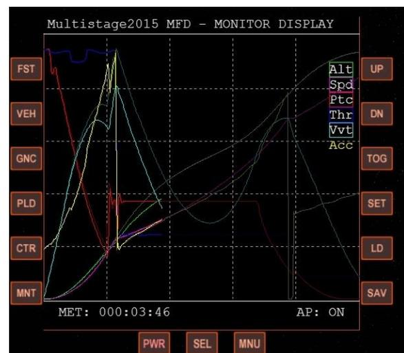
The monitor screen shows live-time graph of most of the parameters of telemetry.
