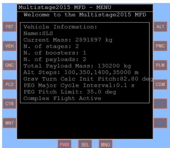
Shows some general vehicle information and gives the possibility to manually set the altitude steps, the Peg Major Cycle Interval, the Peg Pitch Limit and toggles the Complex flight on/off. It also shows the calculated gravity turn initial pitch, for reference if a manual input wants to be set in the guidance program.
