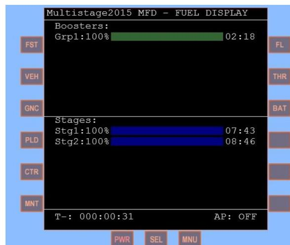
Which shows fuel percentage and time remaining for all the tanks in the rocket.
