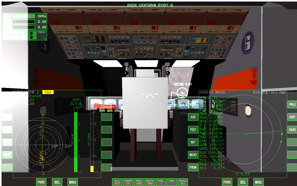
DM Yaw results in Alignment Indicator motion along Dock MFD Y-axis
