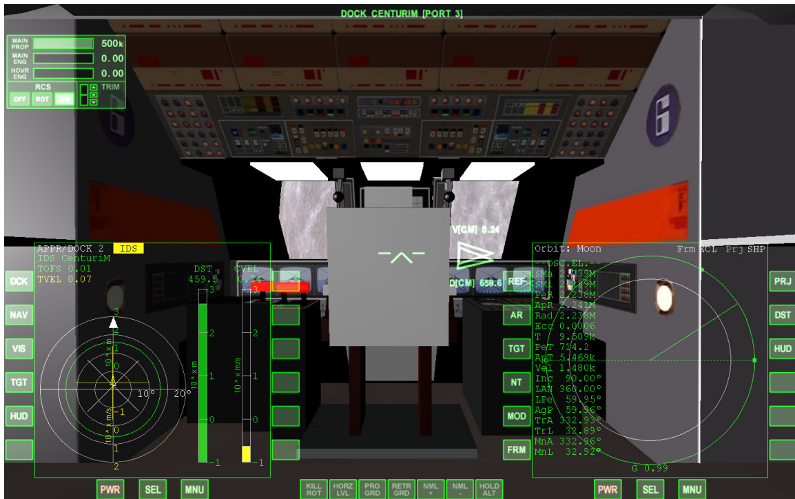
Fwd/Aft translation results in Approach Path Indicator motion along Dock MFD Y-axis
