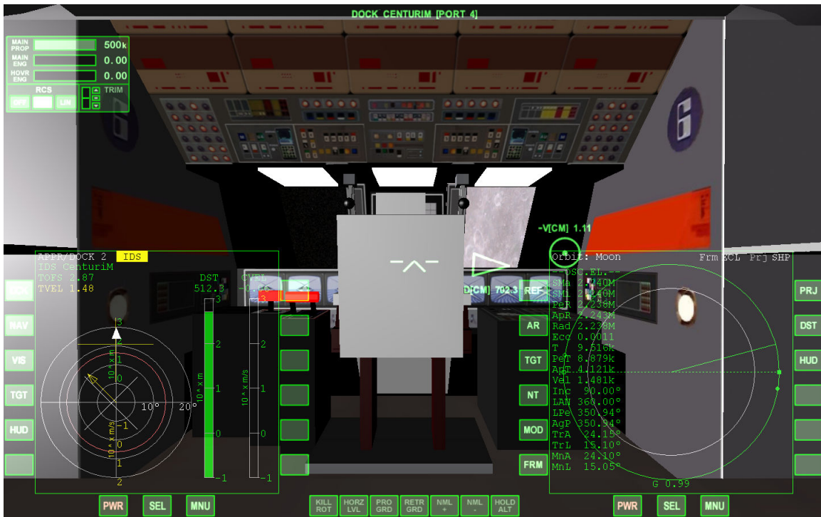
DM Roll results in Alignment Indicator motion along Dock MFD X-axis
