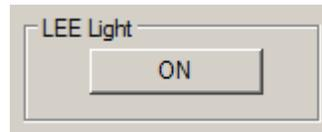
This button allows the user to turn on or off the light associated with the Latching End Effector (LEE) that is NOT attached to the base. Very useful when moving in to grapple an item and the ISS is not in a sun-lit part of the orbit. If the light is "ON", the button displays "ON", if the light is "OFF", the button displays "OFF".
