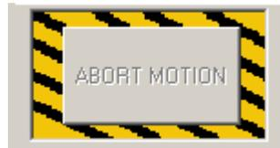
If an auto-sequence move is in progress, the button is enabled. Depressing the button will halt any auto-sequence.
