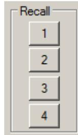
The Recall buttons are only active when there is actually a joint sequence stored in the associated storage location. If the arm is in a “zero-angle” configuration (e.g., all of the joints are at “0” degrees rotation) and that configuration is stored in a location, that location will be considered as empty and the associated Recall button will be “greyed-out” back to an empty configuration.
