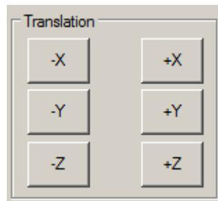
Allows for the inverse-kinematics translation control of the end effector in whichever frame of reference is selected.
