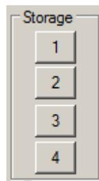
The Storage buttons allow the user to save the current configuration of the various joints for retrieval later in the simulation. If the storage position is not yet used, the associated Recall button is "greyed-out". Saving a configuration into an empty location will cause the associated recall button to become "alive". If a storage location is already used, it can be over-written by pressing the associated location's storage button again.
