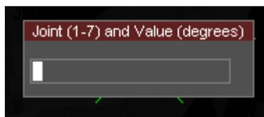
Enter the joint number first, a space, and then the value to set the joint to in degrees (decimals are allowed, so “-189.9” is acceptable). You can continue to use Joint Assign to enter all the relevant joint angles, then when you’ve finished the input, select the Joint Order button and the order for joint movements and the arm will reposition to those values you have input.
