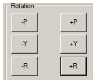
Allows for the inverse-kinematics rotation control of the end effector in whichever frame of reference is selected.
