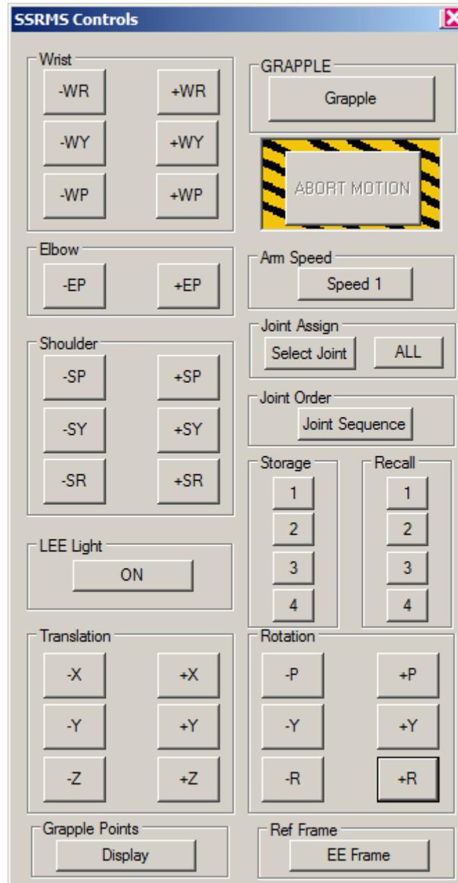
The SSRMS control dialog box can be opened with key sequence “CTRL+SPACEBAR” when the SSRMS is the focus vessel.
