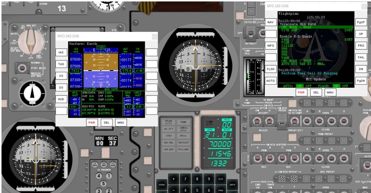
ORB RTE started at DET = 00:00 -> the SRF MDF is in LVLH but FDAI 2 is already not anylonger in 0-0-0 while FDAI 1 (inertial) was almost at 0-0-0 at time ORB RTE was started.
